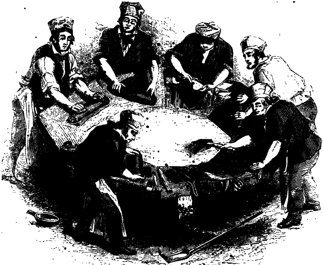
[The Hat Battery, or 'Kenth,' with Men employed in Writing, Rolling, Pressing, 'Rolling,' and Blocking the Hat Bases.]
