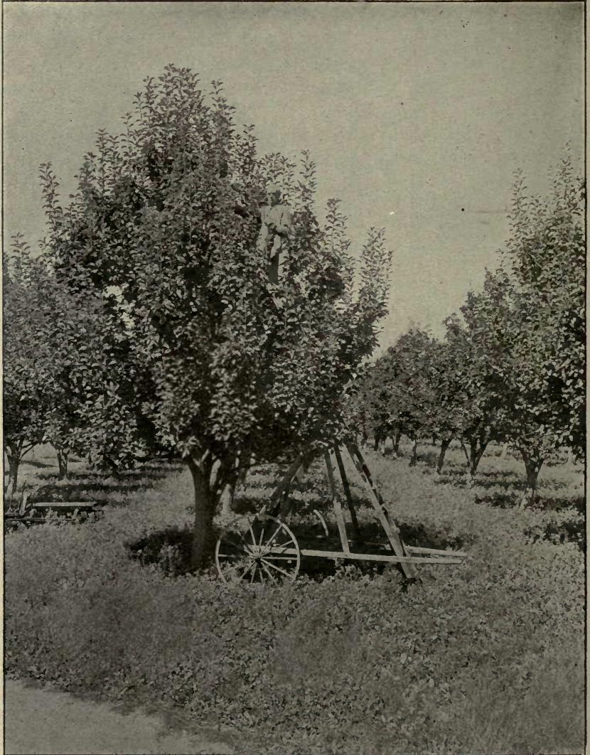
FIG. 300.—WHEEL LADDER FOR PRUNING TREES OR PICKING FRUIT, USED BY L. L. MORRELL, KINDERHOOK, N. Y.
