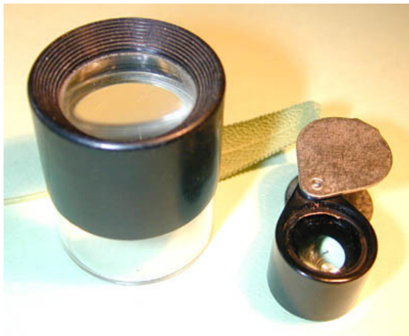
Figure 1 A loupe (left) and a hand-lens (right) - tools used by botanists in the field
