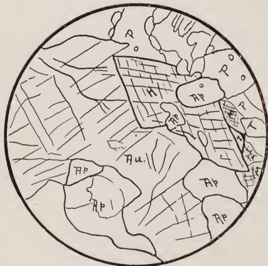
FIGURE 8.— Idiomorphic Hornblende Crystal in the streaked Syenite-gneiss.
