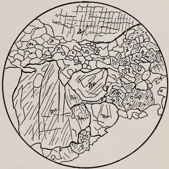
FIGURE 7.—Section transverse to the Pyroxene Band in the ellipsoidal Syenite-gneiss.
