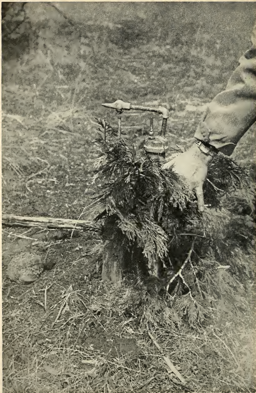
FIGURE 6. Field set of Clover automatic deer marker. Photograph by H. Hjersman, Department of Fish and Game.
