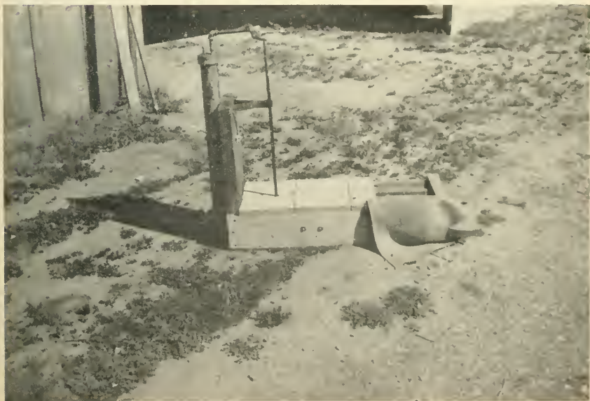
FIGURE 5. Clover automatic deer marker before field setting. Rubber treadle cover removed to show cleats of treadle. Photograph by author.
