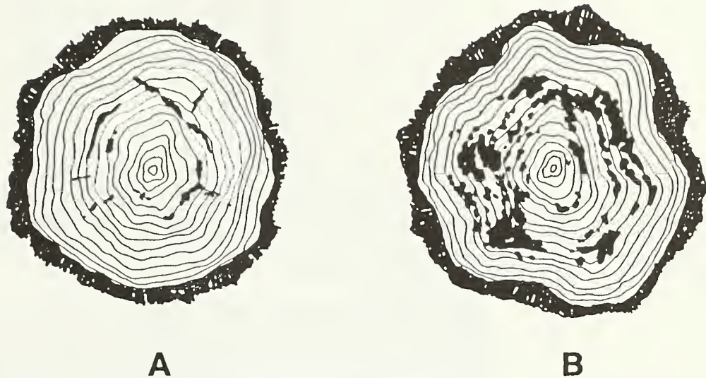
Figure 3—Incense-cedar log ends showing (A) scattered pecky rot typical of the early stages of decay, and (B) large numerous peck holes typical of advanced decay.
