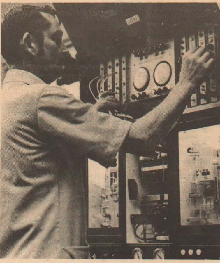
BLOOD TESTER - A machine capable of completing a blood test in 20 seconds is adjusted by HM-1 Don Elam, Senior Hematology Laboratory Technician, NRMC. This new $58,000 Coulter "S" Senior is the most expensive machine used in the lab.
