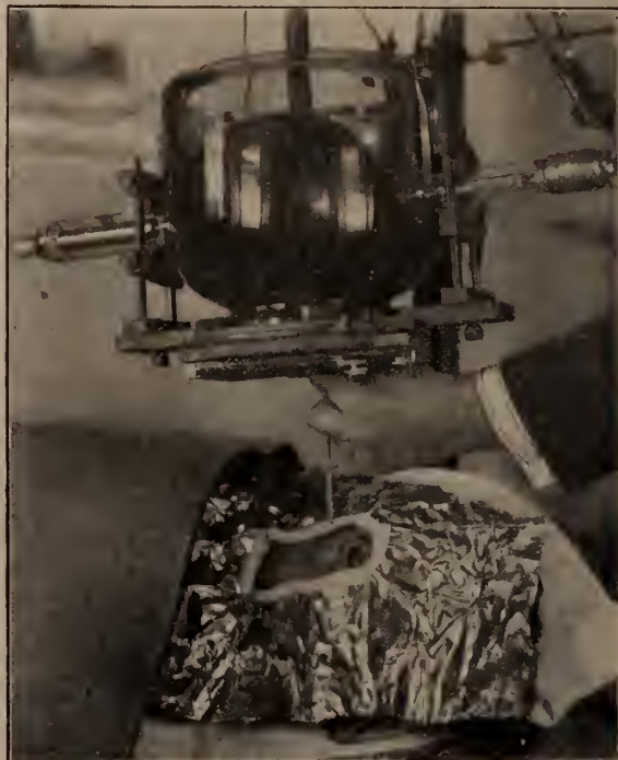
FIG. 1.—Illustrates the use of the indicator in determining the distance and direction of the ray, showing area exposed and position of the patient. Routine factors with this apparatus as follows: Seven-inch spark gap, five milliamperes, ten-inch distance, four minutes' time, with three mm. of aluminum as filter.
