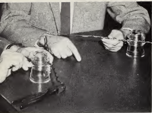
This pre-tied tie was tested at the Bureau laboratories and is now used on rural telephone lines of REA borrowers.
