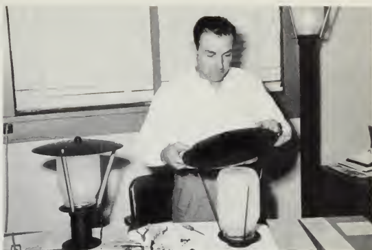
Fitting the shade onto brass tubing over the renovated pickle jar is Assistant Manager Jim Freeman, who designed the yard light.
