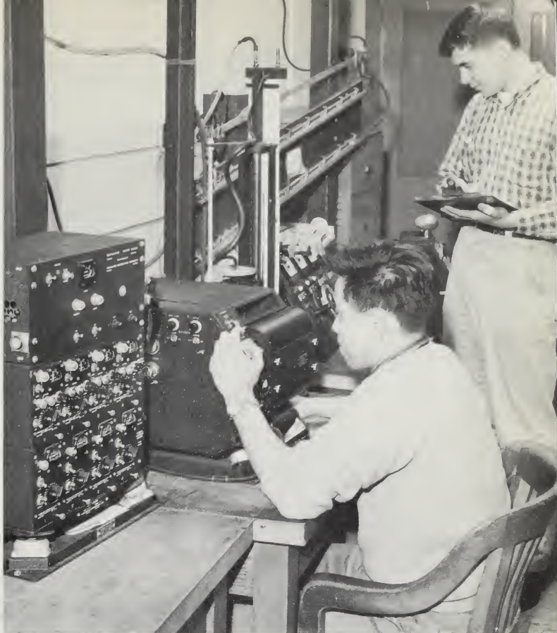
Mechanical engineers of the Bureau adjust oscillographic recorder for a wind tunnel test of wire vibration.
