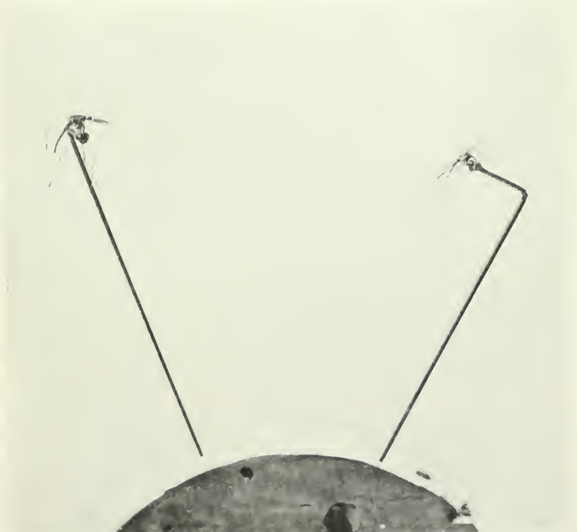
FIG. 2. BLACK ENTOMOLOGICAL PIN WHICH MAY BE STUCK IN CORK AT ANY ANGLE BEST SUITED FOR ILLUMINATION
