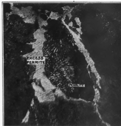
FIG. 1. SLOWLY COOLED CARBON STEEL (B. STOUGHTON)
