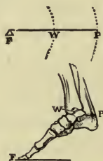
FIG. 118.— Raising Weight of Body upon Ankle. Lever of second order.
