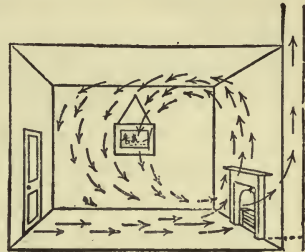
FIG. 150.— Ventilation by an Ordinary Grate or Fireplace. The coldest air chills the feet.
