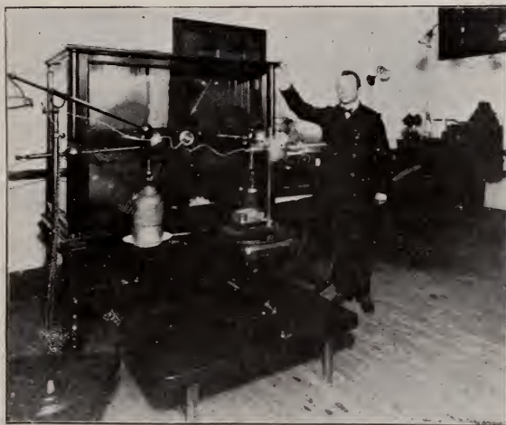
A sixteen revolving plate, Holtz static machine.
