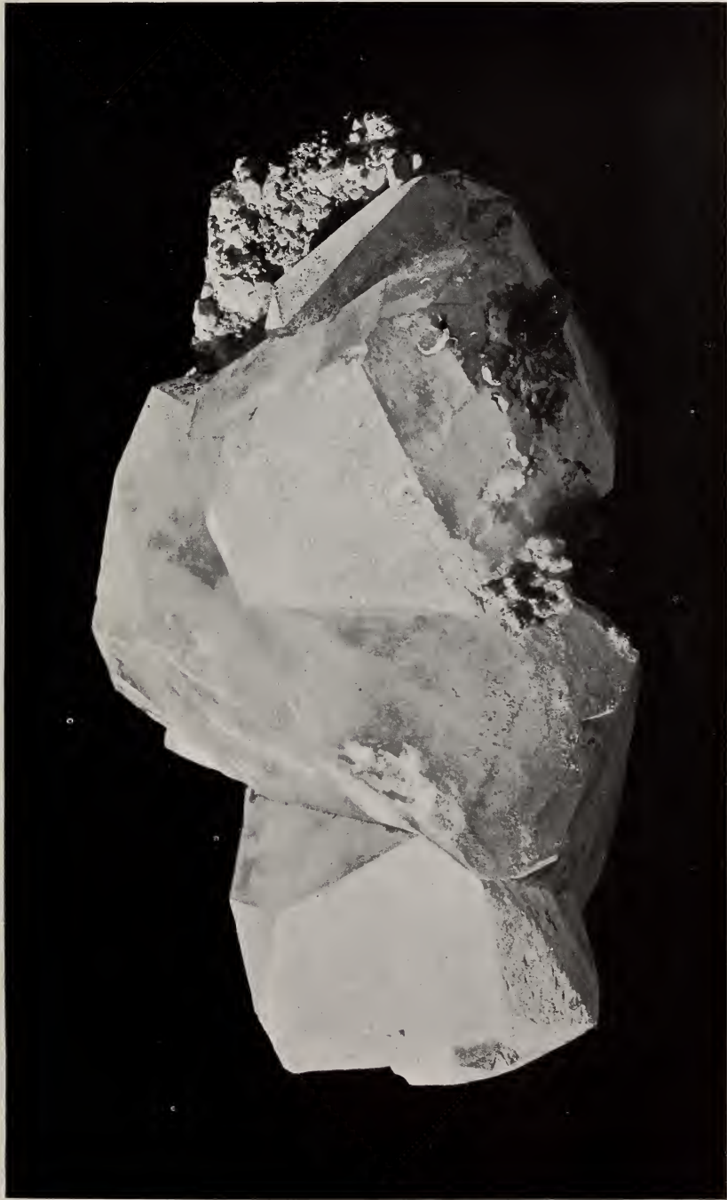
Group of crystals showing repeated twinning parallel to the basal pinacoid which appears in the illustration as a triangular face, the orientation of which corresponds to the two twin positions. The specimen well illustrates the characteristic deep "channels" produced by this law of twinning.
