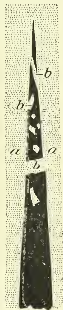
FIG. 31.—Terminal cross section at outcrop of Black Dragon vein, Evacuation Creek. aa , Country. bb , Fragments of wall rock.
