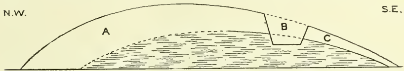
FIG. 40.—Section at Ten Pound Hill, Somerville, Mass., showing drumlin till overlying eroded surface of brick clays. A, thick cobbly till; B, road to Wellington; C, till with striated pebbles seen in clay-pit at this point.
