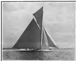
The "Constitution" shortly previous to the Accident The strain of the close-hauled caused the club to bend like a bow, and the mast was taken on, a few moments after came the headwinds.
