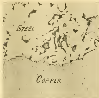
FIG. 1.—Section through a fracture of mild steel, after embedding in an electro-deposit of copper. The path of the fracture among the constituents of the steel can be clearly traced. Magnification, 100 diameters.
