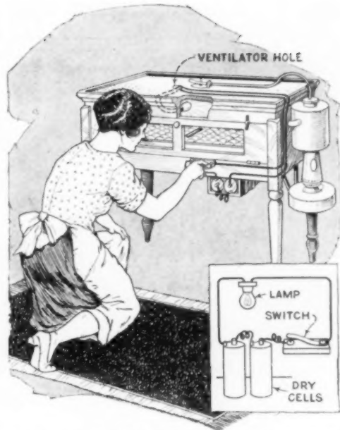
Small Lamp Installed Inside of an Incubator Facilitates Reading the Thermometer
