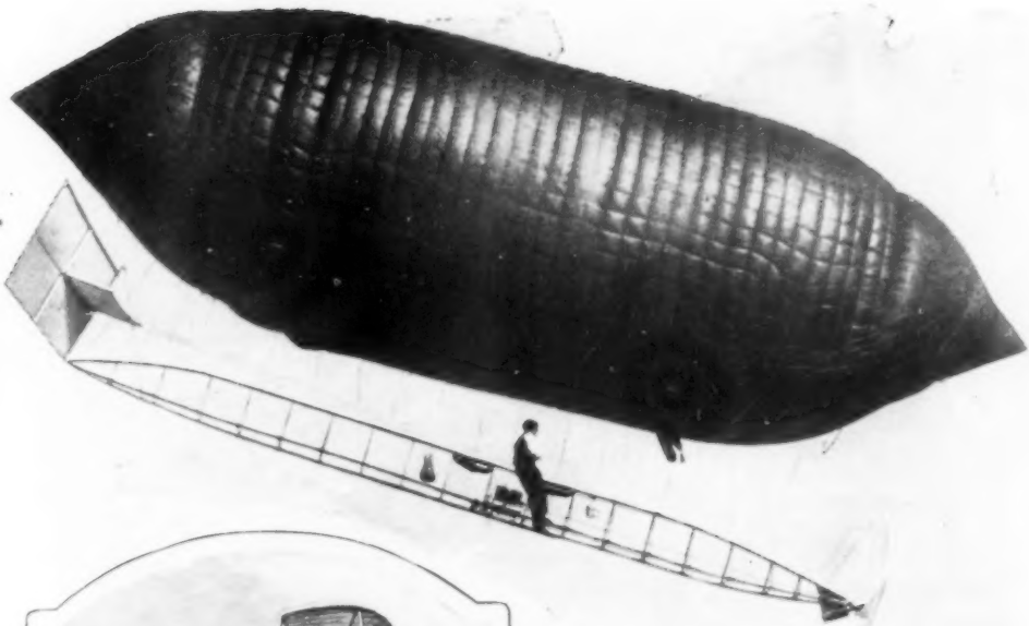
Lincoln Beachey, Later a Famous Airplane Pilot, Got His Start with This Crude Little Dirigible; the Pilot, Straddling a Triangular Frame, Ran Back and Forth along the Keel to Point the Ship Up or Down, as the Bag Itself Had No Elevator Planes; at Left, Wilbur Wright Flying at Le Mans, France; This Is the Plane with Which He Electrified Europe by His Sensational Flights in 1908 and 1909
