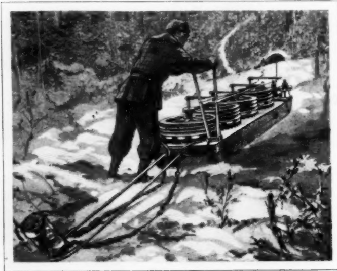
Controlling the Speed of Logs' Descent down Steep Grade with Braking Appliance at the Top of the Hill
