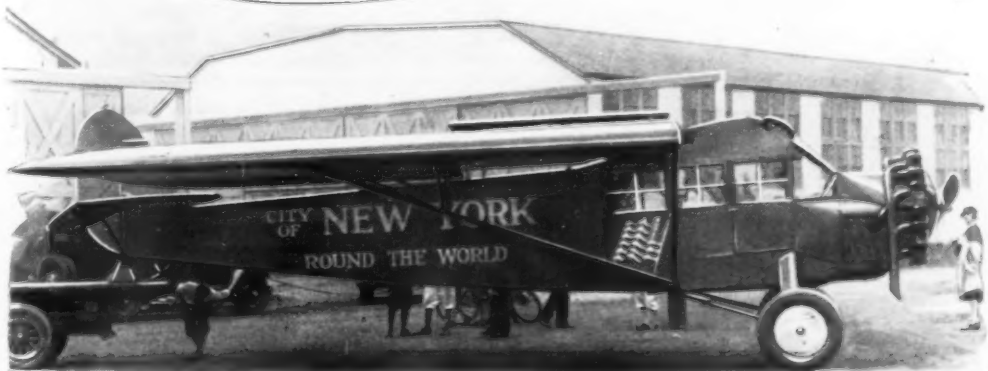
Modern Cabin Plane with Folding Wings; the Fairchild Monoplane John Henry Mears Used in Round-the-World Trip
