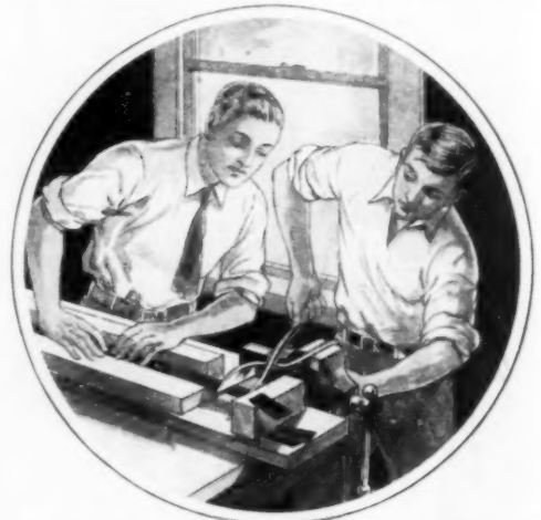
Easy Method of Cutting Transformer Core Strips of Equal Length
