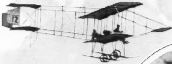
Right, Chinese Military Attache at Washington Learning to Fly; Note the Aileron Controls Strapped to the Shoulders
