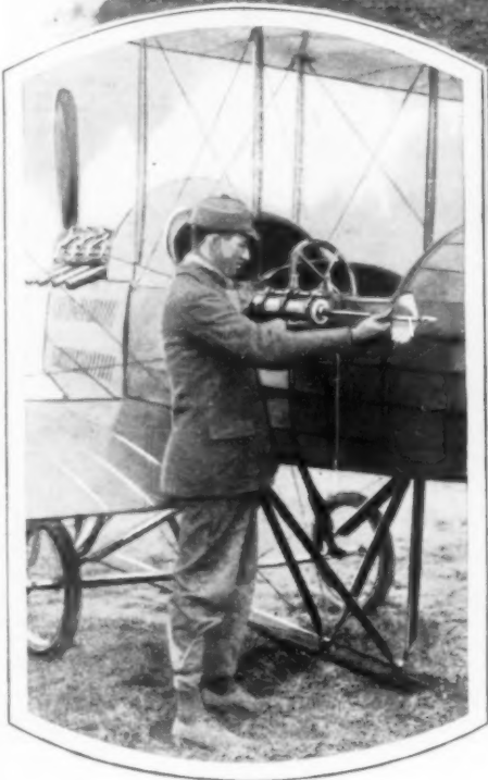
An Early Farman Biplane, of the Days When Planes Still Carried Stabilizers in Front; the Clothes of the Spectators in the Foreground Give a Hint as to the Year; at the Left is the First Aerial Bomb in All History; Its Inventor, Riley Scott, a West Point Graduate, is Attaching the Device to His Plane; the Place is Rockwell Field, San Diego, and the Year is 1913; the Bomb Weighed Six Pounds, in Contrast to the 4,000-Pound Monsters Carried by the Huge Bombing Planes of Today; the Plane Has a Steering-Wheel Control, a Device That is Coming Back into Use for Some of the Bigger Ships Today
