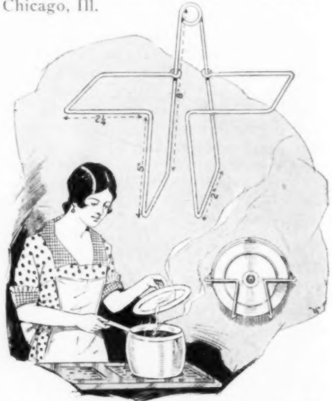
A Length of Galvanized-Iron Wire Makes a Good Pot-Cover Holder for the Kitchen
