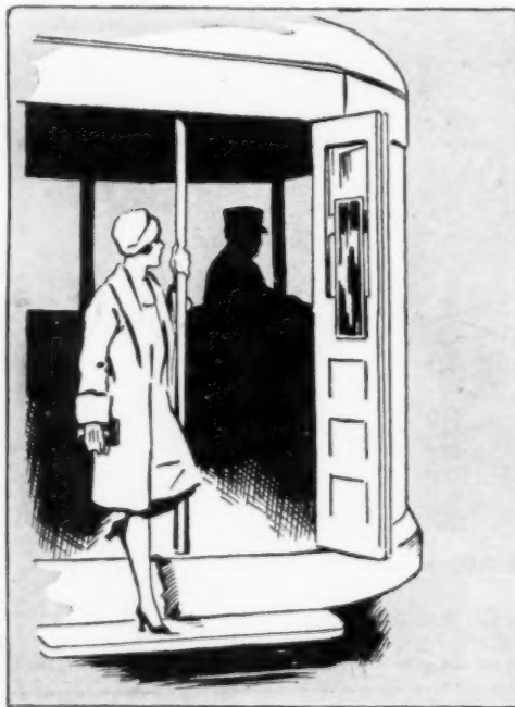
Mirror on Street-Car Exit Door Induces Women to Face Forward When Alighting
