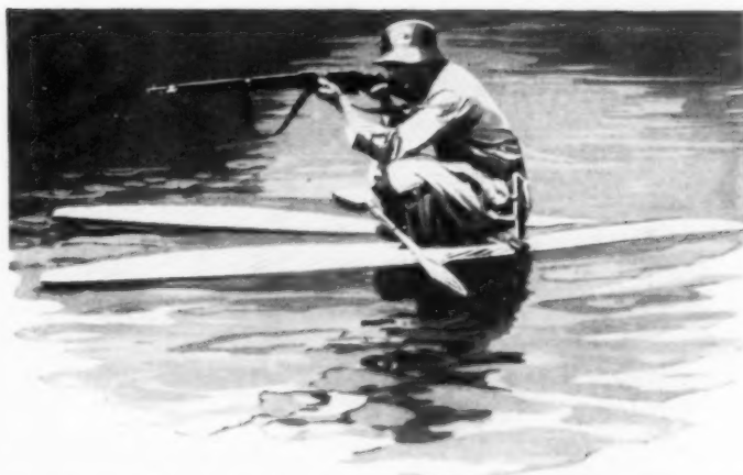
Foot Pontoons for the Soldiers Who Patrol the Danube River; Waterproof Sacks Inside Keep Their Feet Dry
