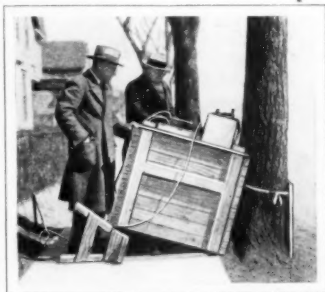
Courtesy Eastman Kodak Co. Taking X-Ray Photo of Tree Interior
