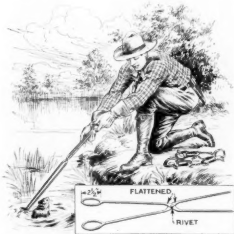
Pair of Tongs Made from Old Hayrake Teeth Useful for Setting Muskrat Traps
