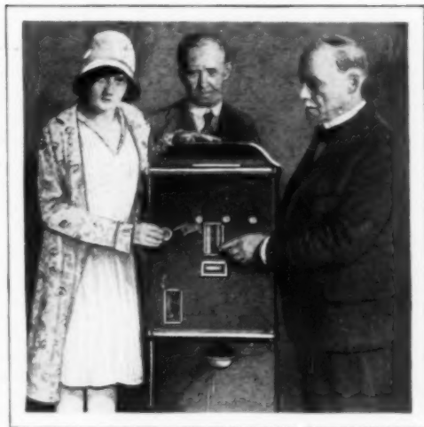
It Functions as a Clerk; Machine That Sells Stamps and Returns the Correct Change
