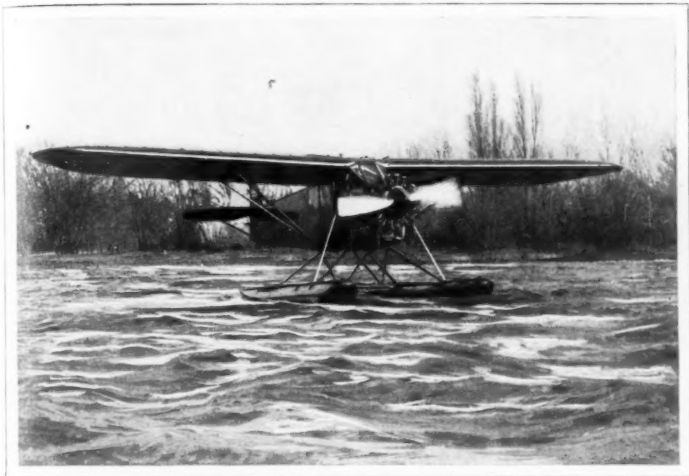
In Summer, Pontoons Replace the Winter Skis; This Is an American-Built Cabin Monoplane with Folding Wings; Wheels Are Never Used in the North as There Are No Landing Fields
