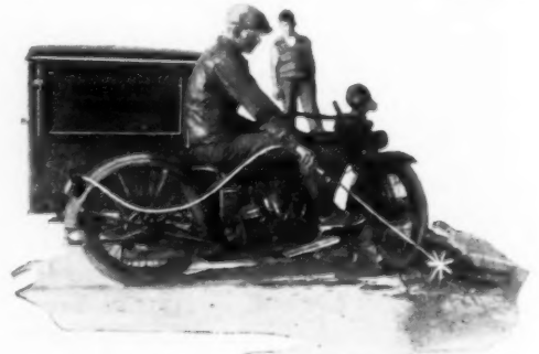
Spraying a Small Pool from the Anti-Mosquito Motorcycle with Its Tank of Tar and Oil
