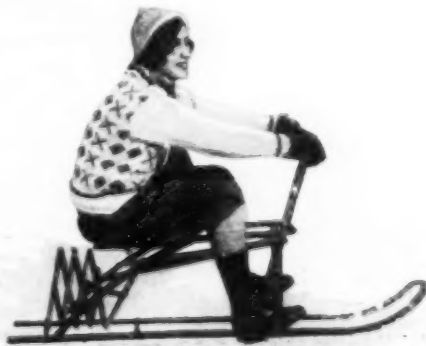
Foot and Hand-Propelled Sled with the "Pusher" Arm at the Rear; Note the Lightweight Construction
