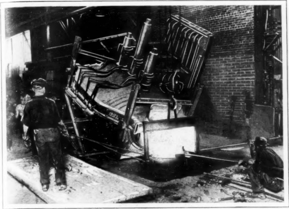
Pouring the Molten Charge from an Electric Steel Furnace; a Large Percentage of All the Energy Generated at Niagara Falls Is Used as Heat in Various Manufacturing Processes
