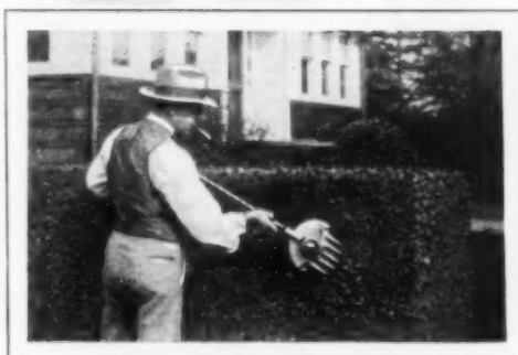
Using the Electric Hedge Trimmer, and Drawings to Show Positions to Which It May Be Adjusted
