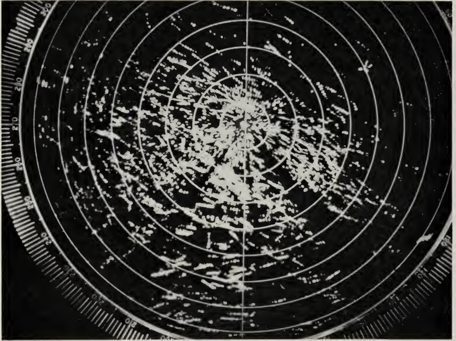
FIG. 2. POW-1 radar screen, Lonely, Alaska, 00:34 ADT, 30 July 1969. Five-minute time exposure, 40 nmi range, echoes moving NW.
