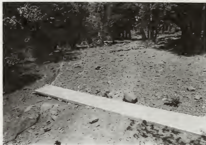
Figure 1.—Looking upslope at an erosion pavement in the ponderosa pine forest. Collector trough with sheet metal borders at each side is in the foreground.
