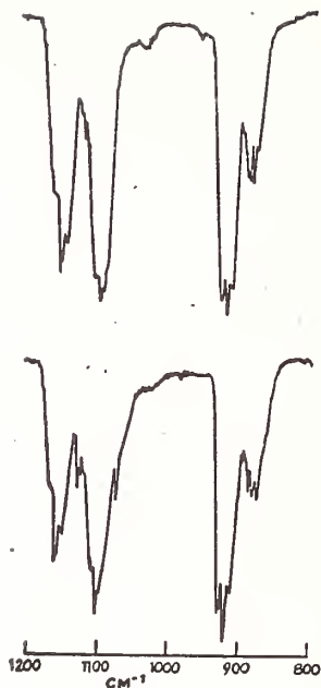
Figure 1. TOP: \text{Cl}_2\text{CF}_2 prior to laser photolysis. Pressure approximately 10 torr. BOTTOM: \text{Cl}_2\text{CF}_2 recovered after laser photolysis in the presence of \text{O}_2 . Pressure approximately 10 torr.
