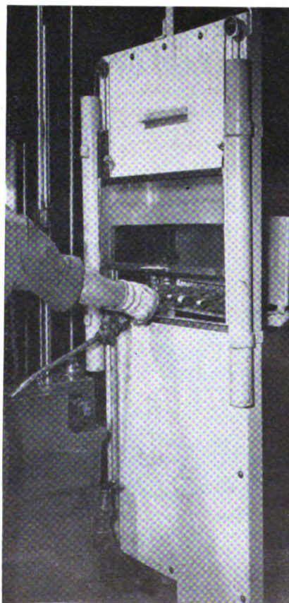
Baffle for control of radiant heat and gas-fired forge.
