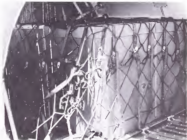
FIGURE 3.—Strawberries assembled on a master pallet, which is set in a forward position in cargo compartment and secured to floor of airfreighter.
