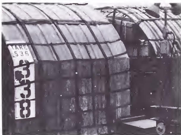
FIGURE 2.—Strawberries on master pallets covered by a fiberglass canopy, or "igloo," ready for loading on airfreighter.
