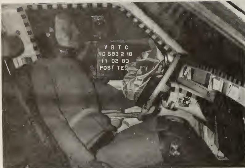
Steering Wheel and Column Damage Test 18
