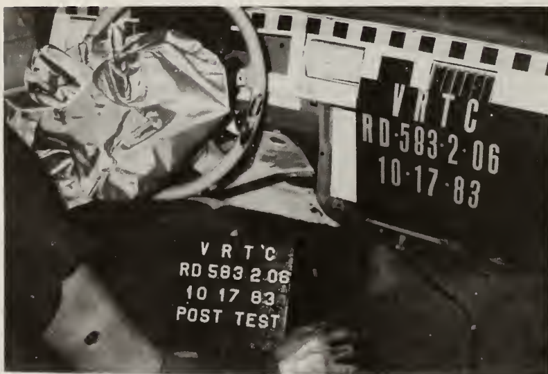
Right Knee Impact Area Post test 6
