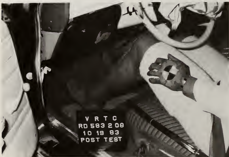
Left Knee Bar Deformation Test 8
