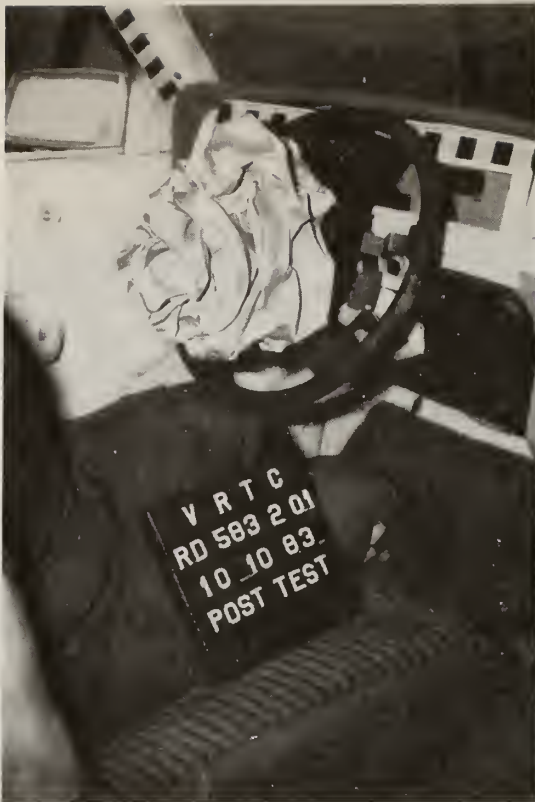
Steering Wheel Deformation Test 1
