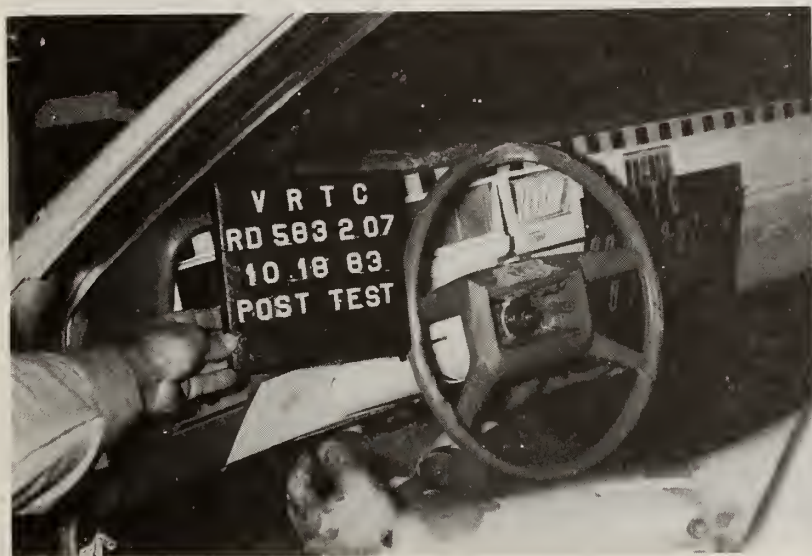
Steering Wheel Deformation, Left View Test 7
