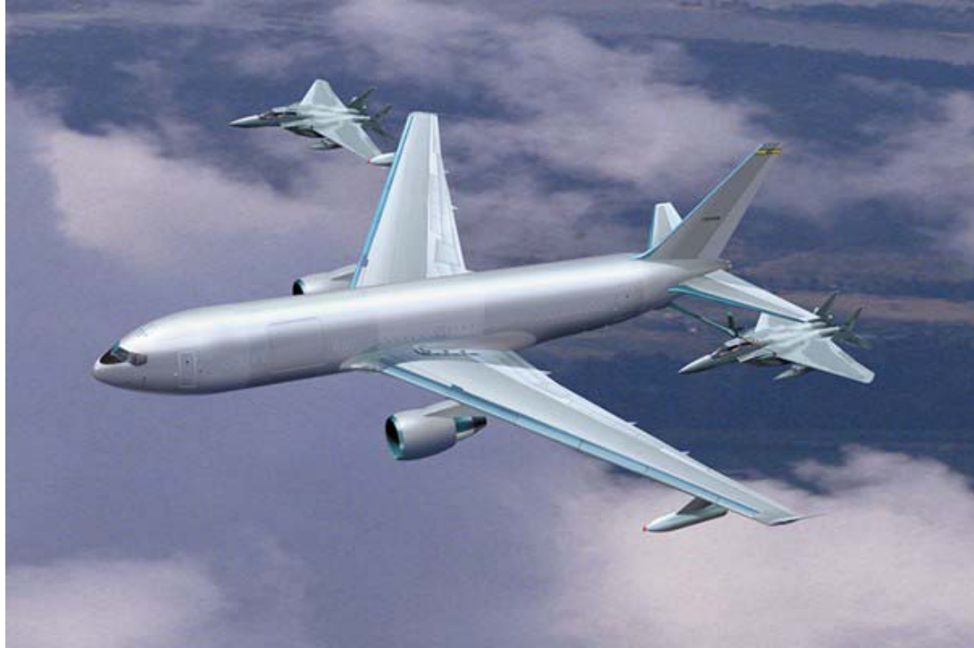
FIGURE 3. BOEING’S RENDITION OF THE KC-767A WITH WING-TIP RE-FUEL PODS (From: The Boeing Company Website, March 2004 )
