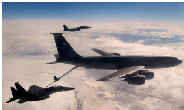
FIGURE 1. KC-135R REFUELING A F-15 WITH THE FLYING BOOM (From: The Boeing Company Website, March 2004 )
