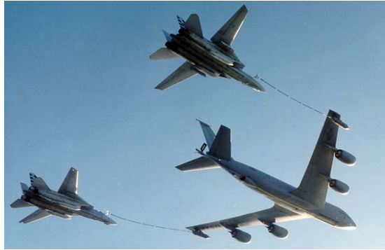
FIGURE 2. KC-135R REFUELING TWO F-14S WITH THE HOSE AND DROGUE SYSTEM
