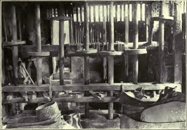
Figure 17. Interior of a primitive rice mill operated by water power.
