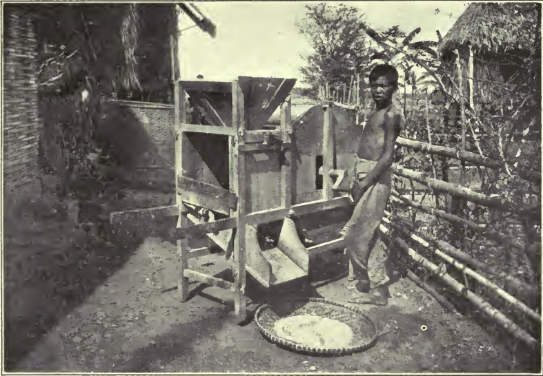
Figure 15. Filipino fanning mill for removing dirt and chaff from rice.
