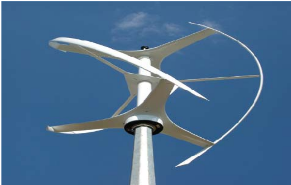
Figure 5. The vertical axis wind turbine. From [7]
