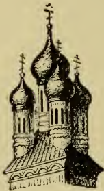
Fig. 111. HIP-ROOF WITH SUPERINCUMBENT DOMES.
