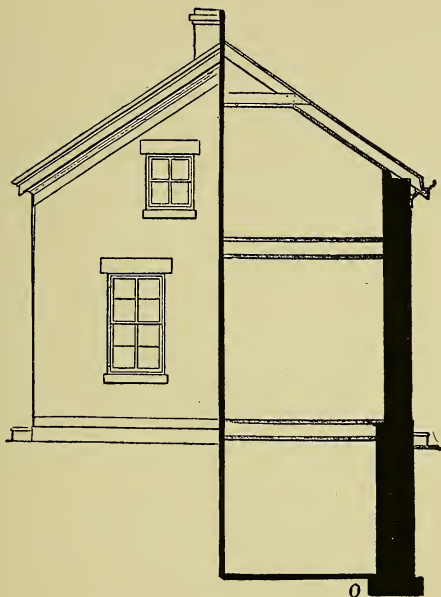
Fig. 104. End Elevation and Section.
