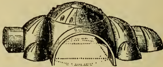
Fig. 89. DOME-SYSTEM OF THE CHURCH OF STA. SOPHIA AT CONSTANTINOPLE.
