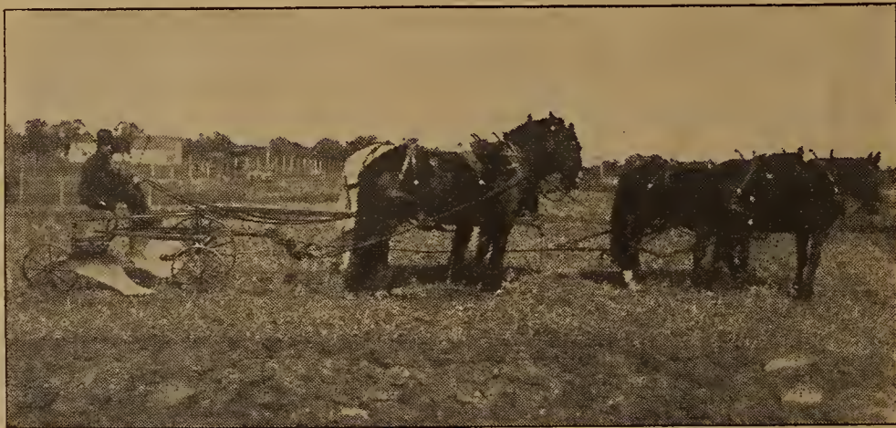
This is a deep-tillage plow in moldboard style. It will plow 16 inches deep. Observe the narrow throat just above the share
