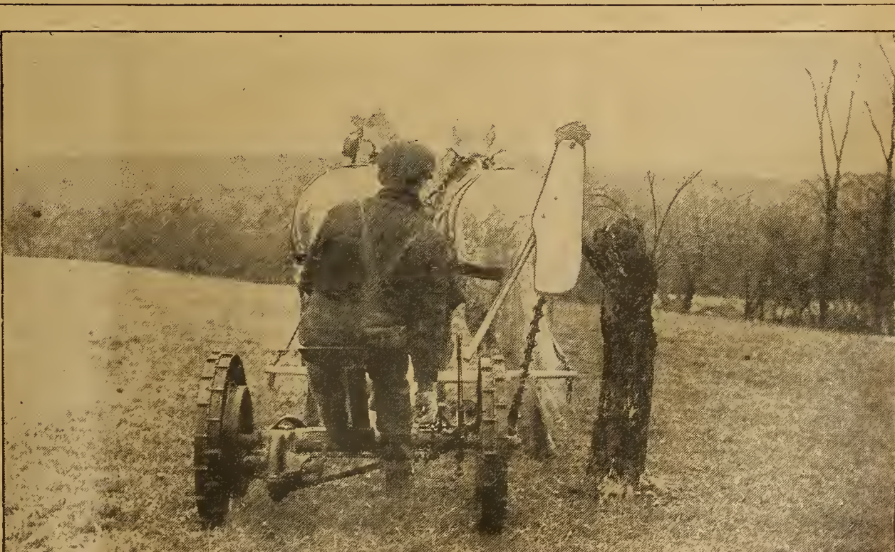
The vertical-lift device for mowers, as shown here, saves time in working among stumps and trees. The driver raises and lowers the cutter bar without leaving his seat
