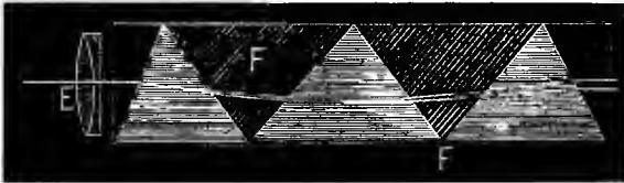
Fig. 69. LENS AND PRISMS FORMING A DIRECT VISION SPECTROSCOPE
