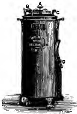
Fig. 28A. ACETYLENE GAS GENERATOR FOR LANTERN WORK.
