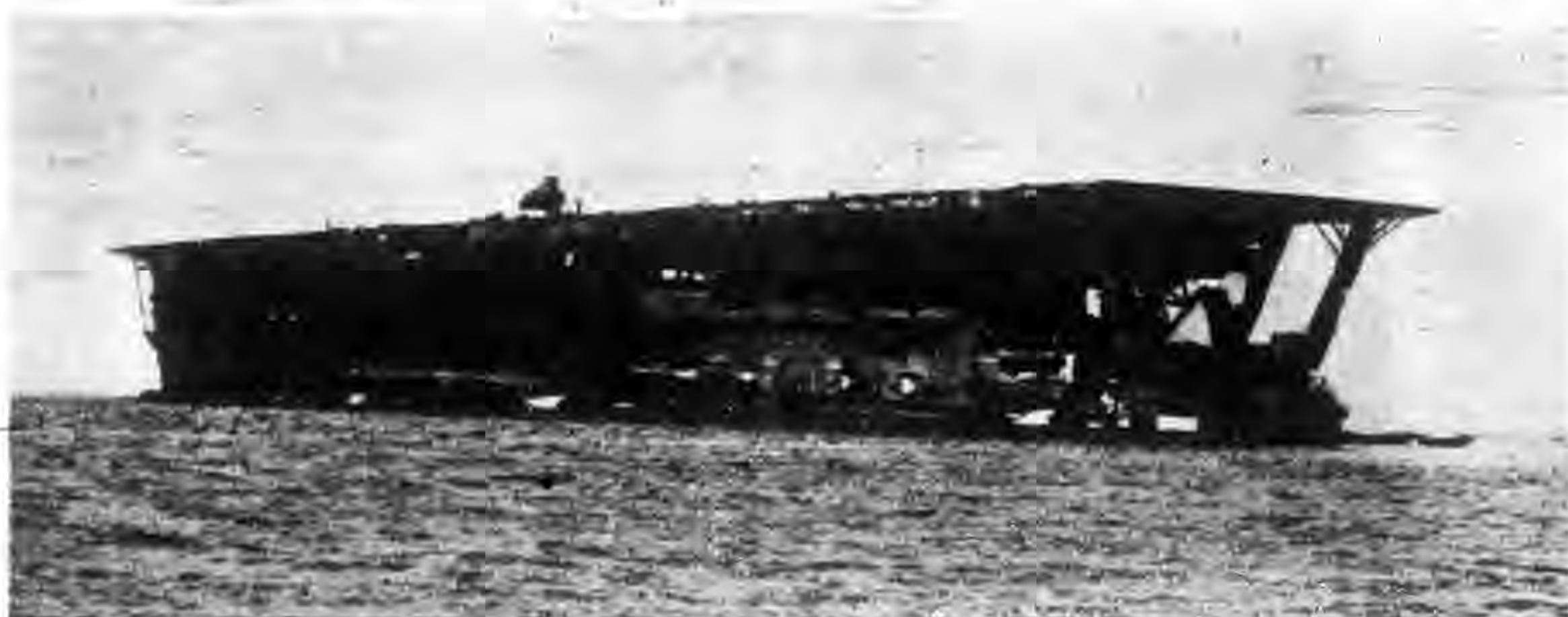
The reconstructed "Kaga": A Japanese aircraft-carrier, originally laid down as a battleship, which has had the flight-deck extended.
