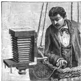
FIG. 3.—Arrangement of photographic apparatus in the balloon.
