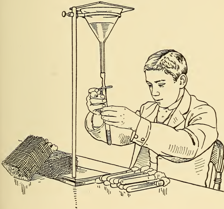
FIG. 16.—Method of filling test-tubes with culture-medium (Warren).
