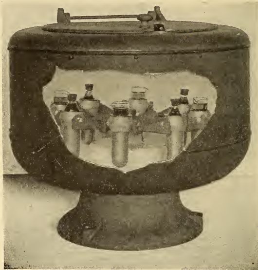
FIG. 7.—Centrifuge, size 1, type B, with 8-tube, 50 c.c. head manufactured by the International Equipment Co.
