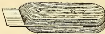
FIG. 2.—Knife for freezing microtome, made from the blade of a carpenter's plane.
