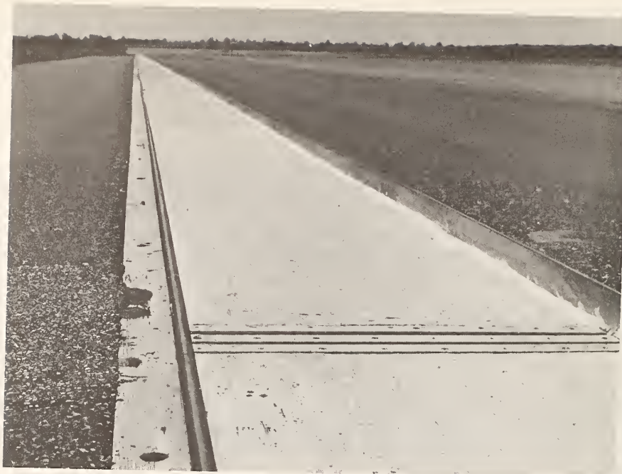
Figure 25. Hydroplaning trough (Water is injected through the slit in the foreground and slowly flows down between the rails.)
