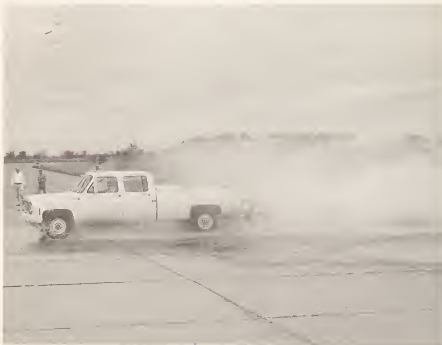
Figure 56. Severe splash and spray (some self-generated) obscuring test trailer
