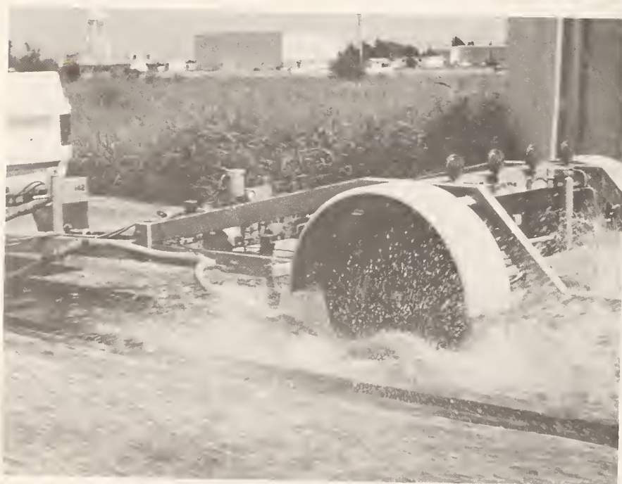
Figure 26. Test run in the hydroplaning trough (The test wheel is offset to allow tow vehicle to straddle the trough.)
