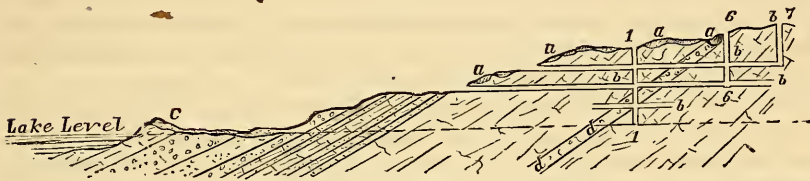
SECTION ON THE COPPER FALLS VEIN. Explanations.— [Hatched pattern] Trap rock. [Dotted pattern] Conglomerate beds. [Stippled pattern] Sandstone.—a a a. Ancient pits on the vein.—b b b. Shafts and galleries of the mine.—c. Sand dunes.—d d. Copper bearing bed of trap.
