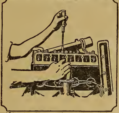
Valves placed in perfect adjustment by turning down ball and socket joint of rocker arm with screw-driver.
