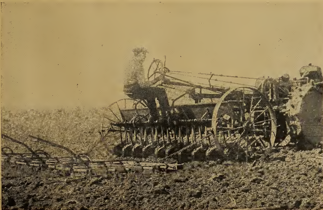
The ability of the tractor to handle several implements at once lowers cost of crop production
