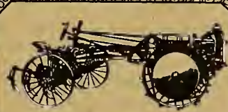
Moline-Universal Two-Row Cultivator —With this outfit 10 to 20 acres a day can be cultivated. Entire outfit easily handled. Tractor speed easily regulated from ½ to 3½ M. P. H. Cultivator is extra strong and has pendulum foot gang shift.
