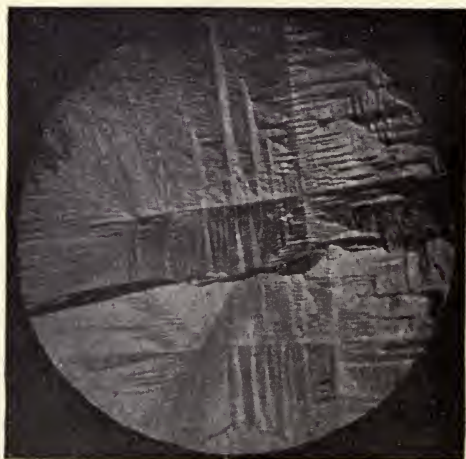
FIG. 76.—Fused Silver. Dendritic Surface ( \times 33 ).
