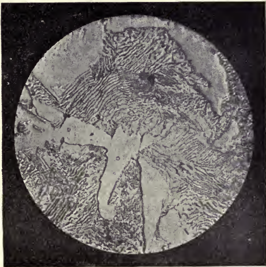
FIG. 178.—White Cast Iron. Cementite (White) with Lamellar Pearlite ( \times 500 ).
