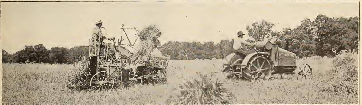
Just an incident of modern farming. Cutting, binding and shocking the wheat in one operation. Two machines, two men, little labor and less worry about it for the farmer. Note how the binder is automatically stacking the sheaves it will presently set up on the ground in a standing shock.
