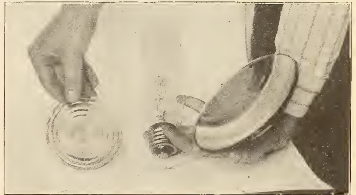
Mirror, lamp and condenser dismantled and displayed. Mirror and condenser are turned to show their faces.
