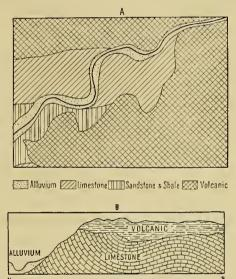
FIG. 166—Geologic sketch map and cross-section in the Cotahuasi Canyon at Cotahuasi. With a slight gap this figure continues Fig. 167 to the left. The section represents a spur of the main plateau about 1,500 feet high in the center of the map.
