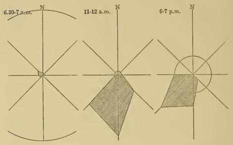
FIG. S8—Wind roses for a station on the eastern border of the Coast Desert near Caraveli during the summer (January to March) of 1913. Compare with Fig. S7. The diameter of the circle in each case represents the proportion of ealm. Note the characteristic morning calm.
