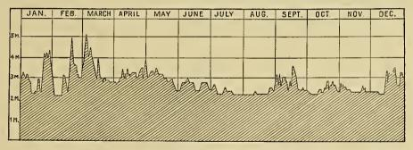
FIG. 70—A stream of the perennial type in the coastal desert of Peru. Depth of water in the Chira River at Sullana, 1905. Data from May to September are approximate. (Bol. de Minas del Perú, 1906, No. 45, p. 2.)
