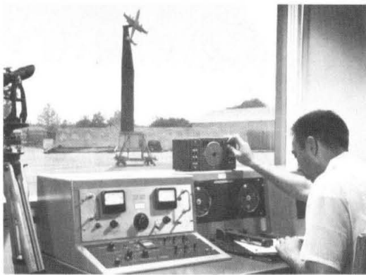
Electronics Research Engineer Irving Alne records radiation antenna pattern on Lockheed's Radar Range. Twenty-two foot plastic tower in background minimizes ground reflections, approximates free space. Pattern integrator, high gain amplifier, square root amplifier and logarithmic amplifier shown in picture are of Lockheed design.
