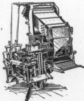
Model 9 quadruple-magazine Linotype, eight of which go into service in the new building.
