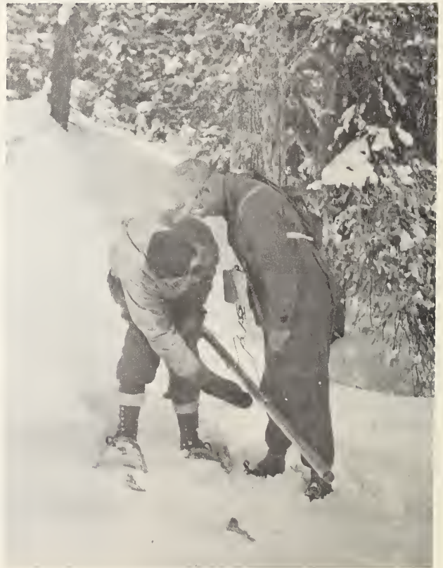
Measuring water content of snow with Utah snow tube
