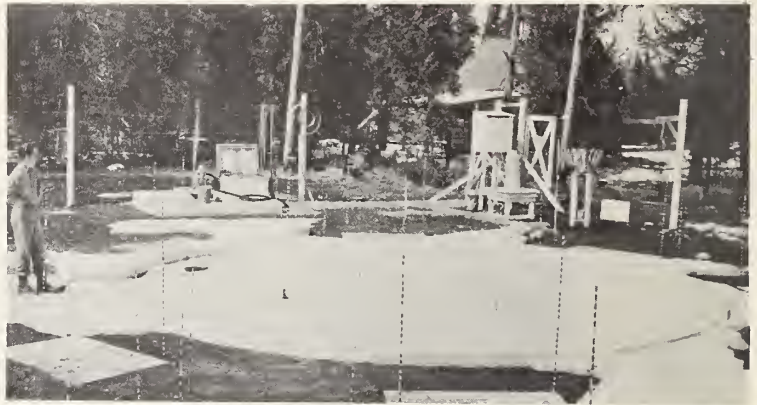
Snow evaporation measured from a 500-square-foot pan
