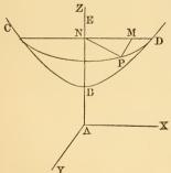
verse axis. Let CBD be an hyperbola, and let it be revolved about its transverse axis BE; then any point on the curve, as D, in its revolution will describe the circumference of a circle. Let the origin be placed at the centre of the hyperbola, and let the transverse axis of the hyperbola be the axis of z.
