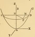
AB; then any point on the curve, as D, in its revolution will describe the circumference of a circle. Let the origin be placed at the vertex of the parabola, and let the axis of the parabola be the axis of z.
