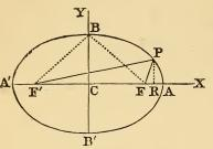
Let F and F' be the foci, and draw the rectangular axes CX, CY, the origin, C, being placed at the middle of FF'. Let P be -X any point of the curve, and draw PR perpendicular to CX.
