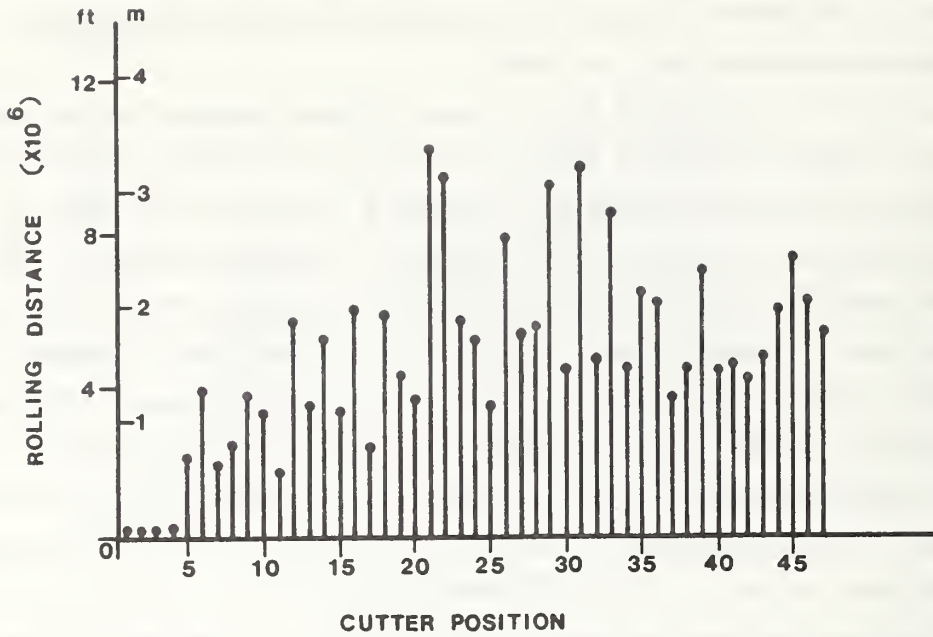
FIGURE 12.7 AVERAGE ROLLING DISTANCE PER CUTTER POSITION, MAIN TUNNEL OF TARP CONTRACT 73-287-2H
