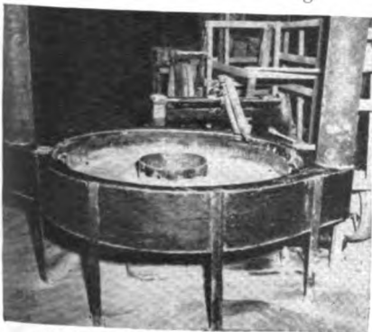
BELOW-1. Ventilated wire panning unit. CENTER-2. Ventilated depanning unit. RIGHT-3. Rotating table and exhausted scoop for pan cleaning.
