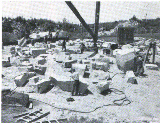
In this concentrated area five pneumatic drills operate in the wet drilling process to completely control dust. The large 25-ton rough blocks on the flat cars are unloaded to be shaped into granite squares and shipped to the finishing plants.
