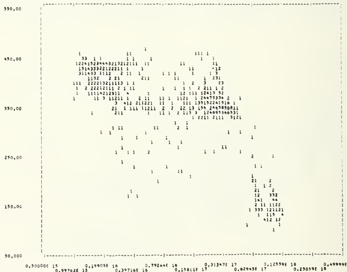
Figure 17. Example of a correlation, or scatter, plot where the field-effect mobility is plotted against carrier concentration.
