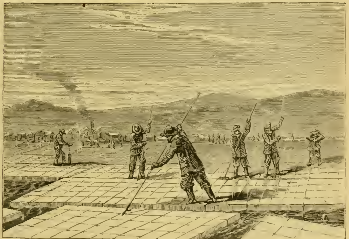
Fig. 3. SAWING AND BARRING OFF.
