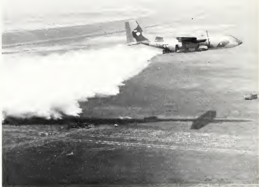
Figure 5.—MBB-firefighting-kit in C-160 Transall in use.
