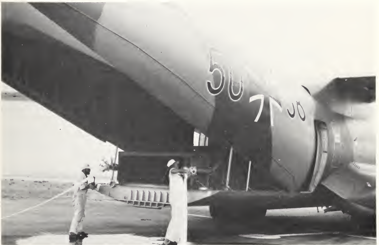
Figure 3.—Installation of MBB-firefighting-kit in C-160 Transall.
