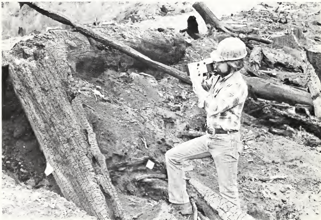
Figure 2.—Using ProbeYE employee is checking a recently completed prescribed burn. Flag markers indicate where hotspots were discovered.
