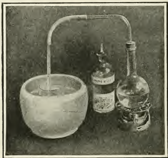
Fig. 187—Apparatus for making synthetic lilac
