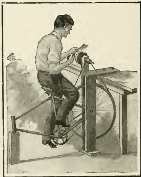
Fig. 29—A simple foot-power grinder
