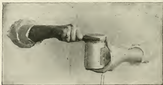
Fig. 294—Unscrewing a tight jar top
