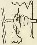
Fig. 8—Tracing a profile of the weather boards
