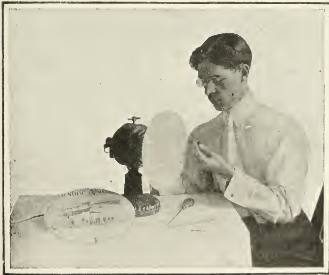
Fig. 180—Cutting a pencil with a disk of Bristol board
