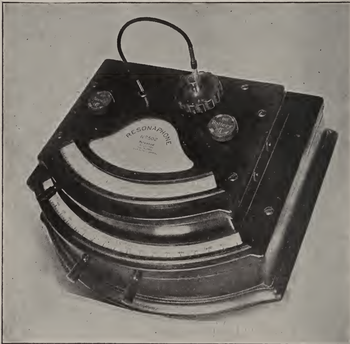
FIG. 13.—DETECTOR MOUNTED ON WAVE METER.
